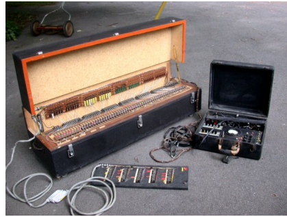
(a) The Vochrome open exposing the row of harmonium reeds.
