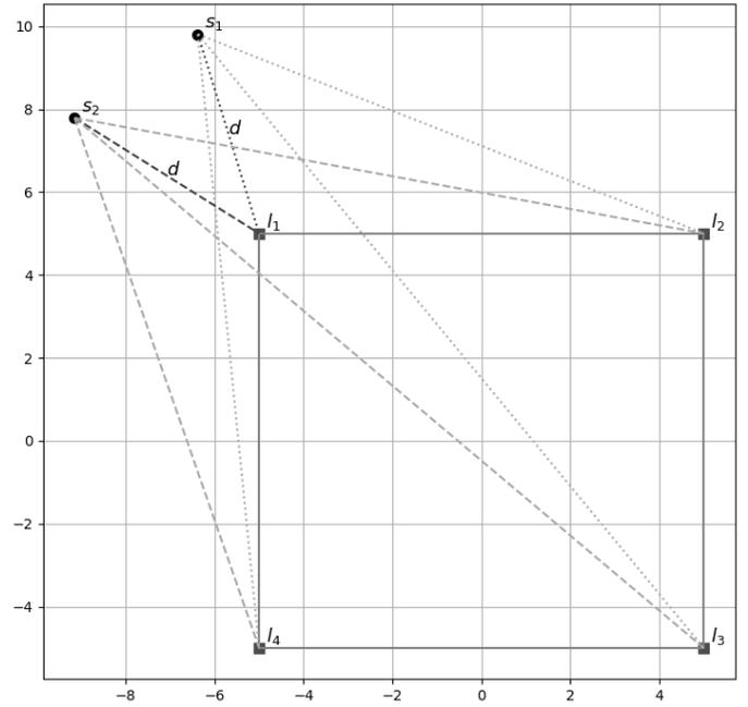
Fig. 1. Both  $s_1$  and  $s_2$  have the same projection,  $l_1$ , and are the same distance,  $d$ , from  $l_1$ . This results in identical gain calculations and therefore, no spatial differentiation. Note, though, that the distance to  $l_2$ ,  $l_3$ , and  $l_4$  are different. When using the original DBAP algorithm, the solutions for  $s_1$  and  $s_2$  are identical and they are perceptibly undifferentiable in space.
