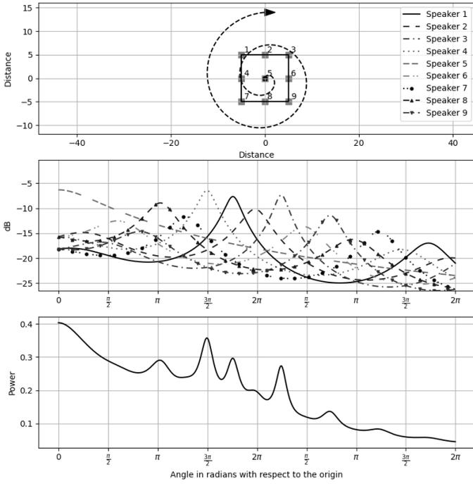
Fig. 4. ADBAP. Rolloff = 6. *Top*: Plot of a 3x3 grid of loudspeakers with a line showing the movement of the source from the center of the field, extending in a spiral to a point outside the field. *Middle*: Gains of the each speaker, color coded to correspond to the above figure. *Bottom*: The power of the entire field as a function of the source’s angle.
