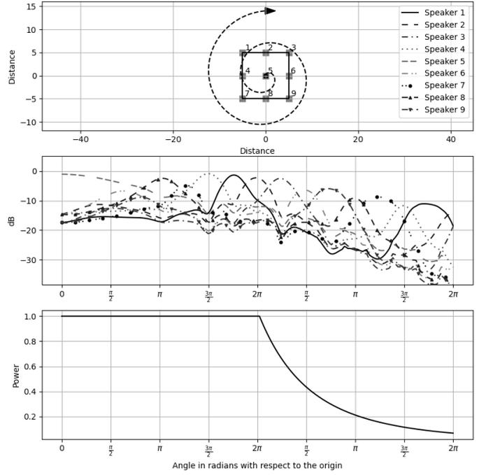
Fig. 3. New DBAP. Rolloff = 6,  $r_s = 1.073$ . *Top*: Plot of a 3x3 grid of loudspeakers with a line showing the movement of the source from the center of the field, extending in a spiral to a point outside the field. *Middle*: Gains of the each speaker, color coded to correspond to the above figure. *Bottom*: The power of the entire field.
