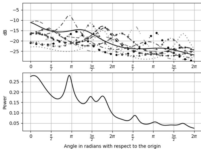
Fig. 7. Gain curves for ADBAP. Although the behavior is much more what is expected, note the spike in power around the first  $\pi$  when the virtual source closes in on the cluster of speakers 2 and 8.
